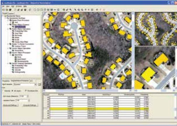
The IMAGINE Objective user interface showing a feature model designed to extract the locations of building footprints in a GIS-ready form to minimize manual post-processing and editing.
